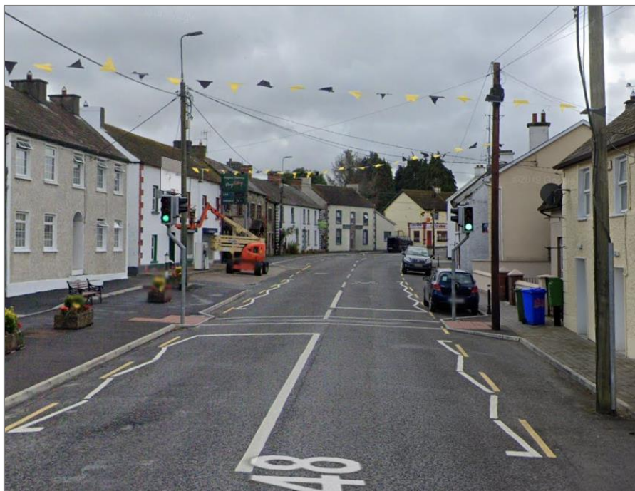
Figure 15-6 - Signalized Pedestrian Crossing in R448
