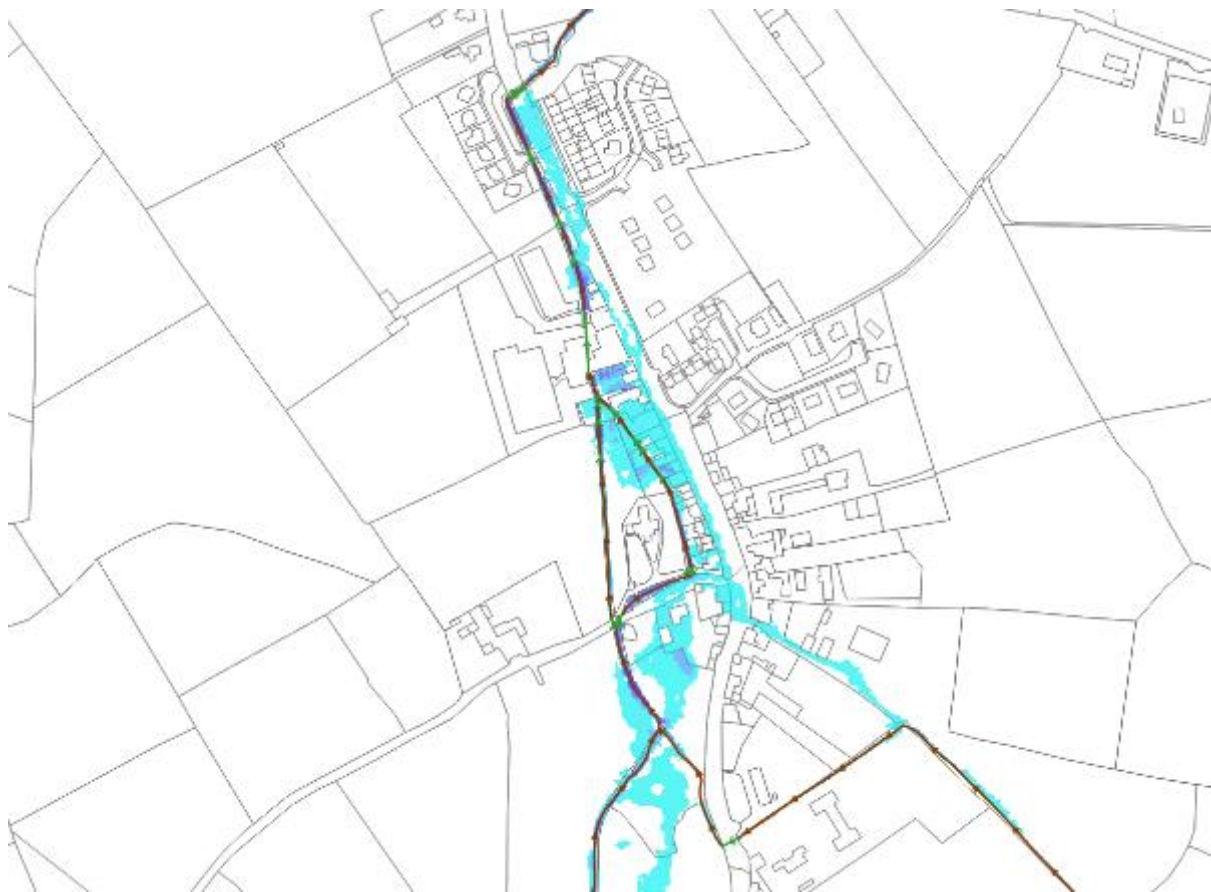
Figure 5-3 Fluvial Flood Extents 1% AEP (Source – McCloy Consulting – Hydraulics Report Ballyhale, Co. Kilkenny)
